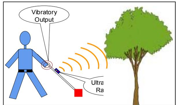
**FIGURE 2: ULTRASOUND BASED RANGING COMBINED WITH VIBRATORY OUTPUT**
