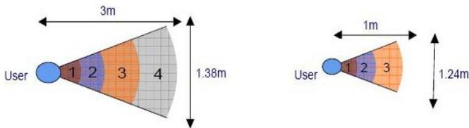
**FIGURE 5: TOP VIEW SHOWING THE HORIZONTAL AND ANGULAR COVERAGE OF THE DETECTION ZONE (COLORED) FOR LONG RANGE MODE (LEFT) AND SHORT RANGE MODE (RIGHT)**
