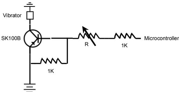
**FIGURE 7: VIBRATOR INTERFACE WITH THE MICRO-CONTROLLER**
