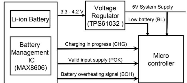
**FIGURE 8: MAX8606 INTERFACE WITH THE MICRO-CONTROLLER**
