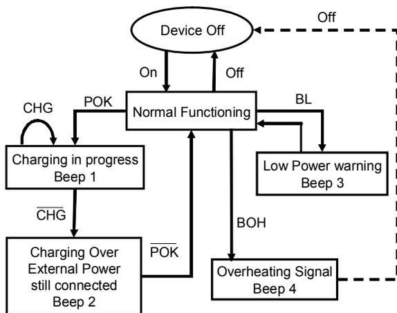
**FIGURE 10: SYSTEM STATE DIAGRAM**
