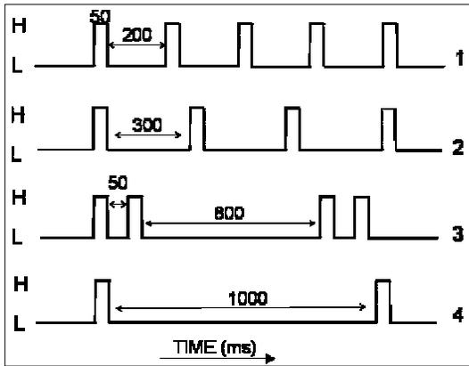
**FIGURE 6: PICTORIAL REPRESENTATION OF VIBRATORY PATTERNS. (H INDICATES THAT THE MOTOR IS ACTIVE WHEREAS L SIGNIFIES NON-VIBRATING INTERVALS)**
