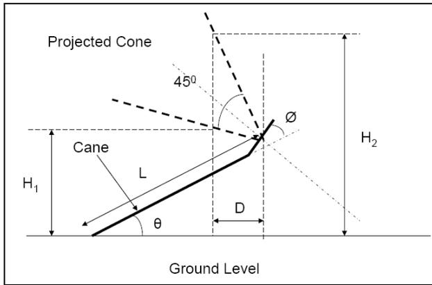
**FIGURE 12: ORIENTATION DETAILS OF SONIC SENSOR**
