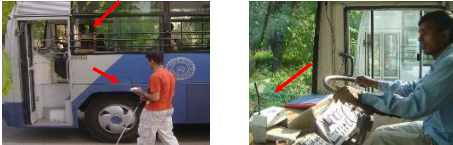
Figure 5: (Left) Bus module installed near driver's controls. (Right) Visually impaired person uses the user module to identify desired bus by triggering auditory cues at the entry of the bus. The person boards the bus independently without any external sighted assistance.
